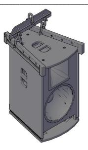
Install BUMPER SF15 and connect it with the LIFTBARs using four GRILLO16. Another GRILLO16 can be used to hook the BUMPER.
