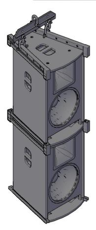
For suspended installation in vertical configuration, mount the ALUBAR in the cases of speakers.
