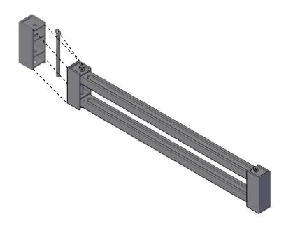
It is possible to install a maximum of three speaker in horizontal configuration and three in vertical configuration.
