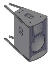
Insert ALUBAR SF15 in the guide slots on the sides of the case. If one speaker must be mounted, insert only the ALUBAR in the upper side.
