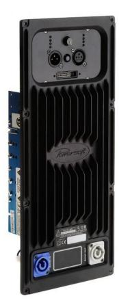
Before making connection between mixer and active speaker, make sure all the switches of the speakers are turned off and the mixer volume is turned down. To avoid a sudden signal, making connection, then turn on the mixer first and then the speakers. Turn on the amplifier by the power switch to position 1 (on).
